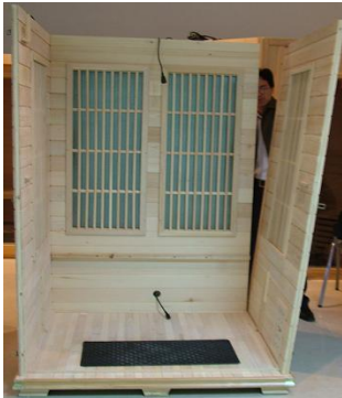
FIG-7 Assembling right board
