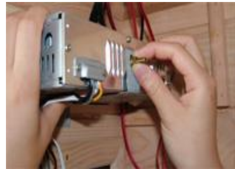
FIG-16.3 Lock the CD with its metal support
