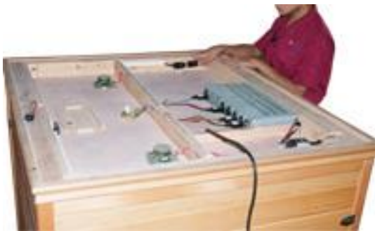
FIG-14 Connectors on the internal top board
