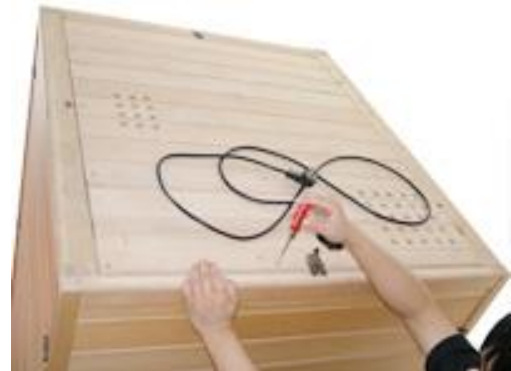
FIG-23 Fix the external board with screws
