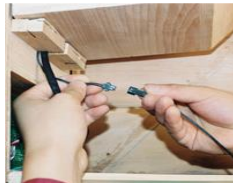
FIG-18 Link the sensor connectors
